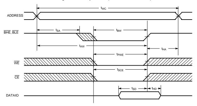
Figure 8. Write Cycle No. 3 (WE Controlled, OE HIGH During Write)[19, 20]
